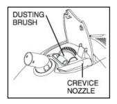
Attach crevice nozzle to the end of the hose for detail cleaning. Attach dusting brush to the end of the hose for dusting.
